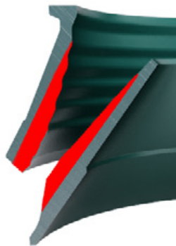
Example of normal wear. Obtained with correct feed arrangements, feed gradation and parameters for the cavity.
